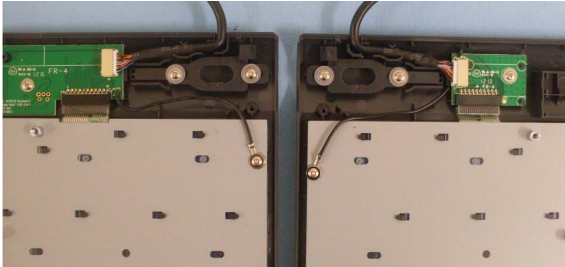
Figure 3. Closeup, showing proper routing and connection of cables.
